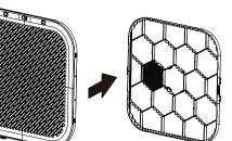
Separate the frame from the filter assembly.
